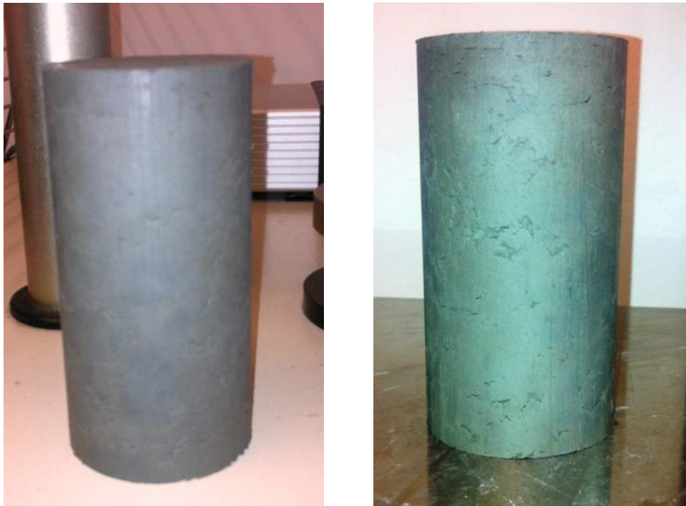
(a) Figure 11: Laboratory-mixed samples before testing (a) 5 m depth (b) 7 m depth
